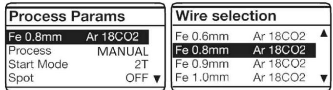
Note: the synergic curves indicated with the acronym **KOP** allow welding with **low heat input**.
