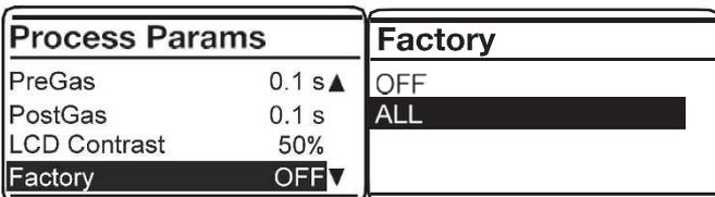
**NOTE.** For all the functions adjusted by means of the adjustment bar, the initial default value can be reset. This operation be performed by pressing the knob **A** for more than 2 seconds only once the adjustment bar appears on the display screen **B**. (Arc Length - Spot Time - Pause Time - Inductance, Burnback – Soft Start - Pre Gas - Post Gas - LCD Contrast).
